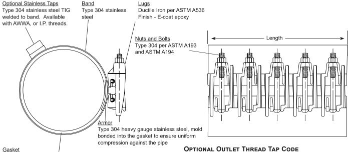
Gridded Virgin SBR compounded for water service per ASTM D2000. NBR (Buna-N) and EPDM are optional.
