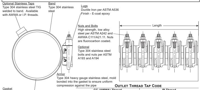
Gridded Virgin SBR compounded for water service, per ASTM D2000. NBR (Buna-N) is available.
