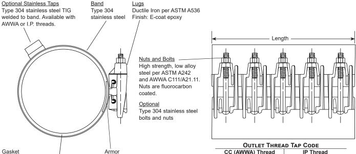
Type 304 heavy gauge stainless steel, mold bonded into the gasket to ensure uniform compression against the pipe
