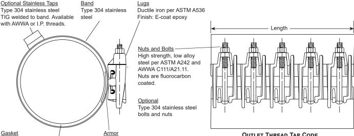
Type 304 heavy gauge stainless steel, mold bonded into the gasket to ensure uniform compression against the pipe
