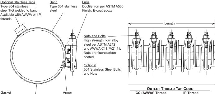
Gridded Virgin SBR compounded for water service, per ASTM D2000. NBR (Buna-N) is available as optional material.
