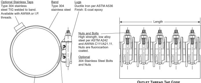
Gridded Virgin SBR compounded for water service, per ASTM D2000. NBR (Buna-N) is available as optional material.
