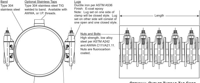
Gridded NBR (Buna-N) compounded for water service, per ASTM D2000.
