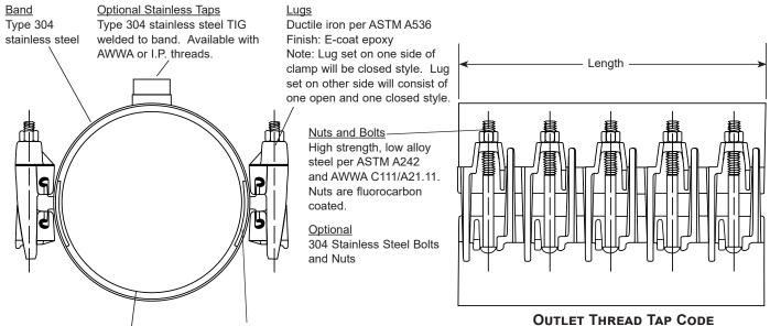
Gridded Virgin SBR compounded for water service, per ASTM D2000.
