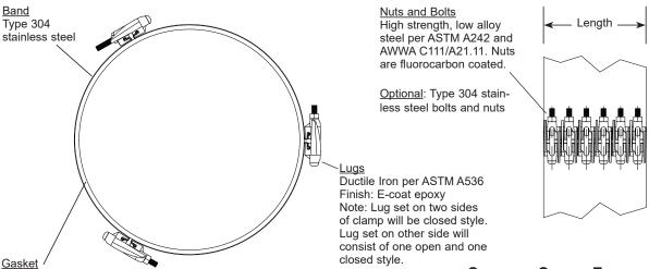
Gridded Virgin SBR compounded for water service, per ASTM D2000. NBR (Buna-N) and EPDM are optional.
