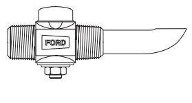
AWWA/CC TAPER THREAD INLET BY MALE IRON PIPE THREAD OUTLET
