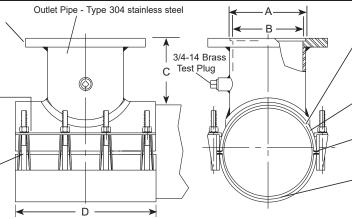
Outlet Gasket - Virgin EPDM compounded for water service, per ASTM D2000. Outlet gasket assures complete seal of outlet area.
