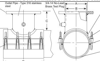
Outlet Gasket - Virgin NBR (Buna-N) compounded for water service, per ASTM D2000. Outlet gasket assures complete seal of outlet area.
