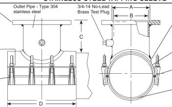
Outlet Gasket - Virgin NBR (Buna-N) compounded for water service, per ASTM D2000. Outlet gasket assures complete seal of outlet area.
