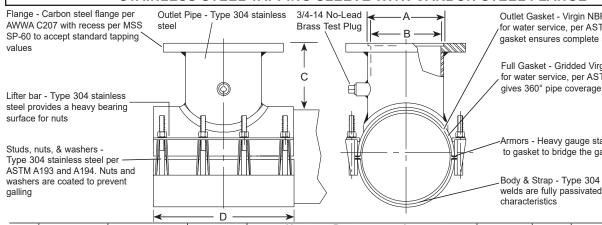
Outlet Gasket - Virgin NBR (Buna-N) compounded for water service, per ASTM D2000. Outlet gasket ensures complete seal of outlet area
