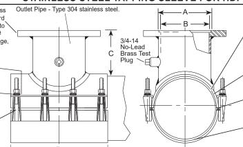
Outlet Gasket - Virgin NBR (Buna-N) compounded for water service, per ASTM D2000. Outlet gasket ensures complete seal of outlet area.
