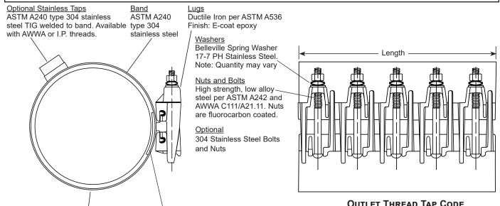
Gasket Gridded Virgin SBR compounded for water service, per ASTM D2000. NBR (Buna-N) and EPDM are available as optional materials.
