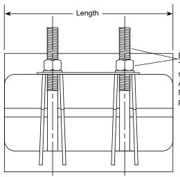
**Bolts & Nuts** Type 304 stainless steel per ASTM A193 and A194. Nuts are coated to prevent galling.
