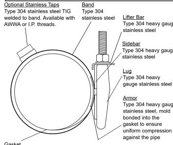
Gasket Gridded virgin SBR compounded for water service, per ASTM D2000. NBR (Buna-N) Nitrile is optional.
