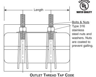
CC (AWWA) THREAD **IP THREAD** CODE NUMBER THREAD THREAD CODE No. 3/4" CC 3/4" IP -IP3 -CC3 1" CC -CC4 -IP4 1" IP 1-1/4" CC -CC5 1-1/4" IP -IP5 1-1/2" CC 1-1/2" IP -CC6 -IP6 2" CC -CC7 2" IP -IP7
