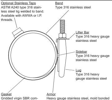
Heavy gauge stainless steel, mold bonded into the gasket to ensure uniform compression against the pipe
