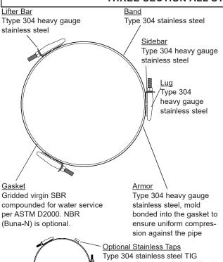
**Bolts & Nuts** Length Type 304 stainless steel nuts and washers per ASTM A193 and A194. Nuts are coated to prevent galling.
