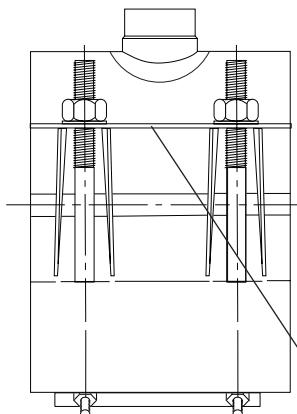
Stainless Steel Nuts and Bolts - Type 304 stainless steel nuts and bolts per ASTM A193 & A194. Nuts are EPIII coated to prevent galling and bolts are MIG welded to side bar.
