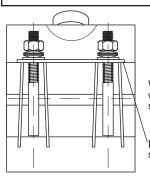
Stainless Steel Nuts and Studs - Type 316 stainless steel per ASTM A193 and A194. Heavy hex nuts are coated to prevent galling.
