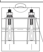
Stainless Steel Nuts and Studs - Type 304 stainless steel per ASTM A193 and A194. Heavy hex nuts are coated to prevent galling.
