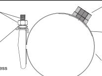
Stainless Taps - Type 304 stainless steel TIG welded to shell. Available with AWWA, FIP 1/2" thru 2".
