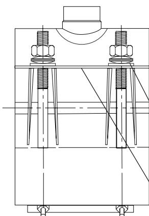
Stainless Steel Nuts and Bolts - Type 304 stainless steel nuts and bolts per ASTM A193 and A194. Nuts are EPIII coated to prevent galling and bolts are MIG welded to side bar.
