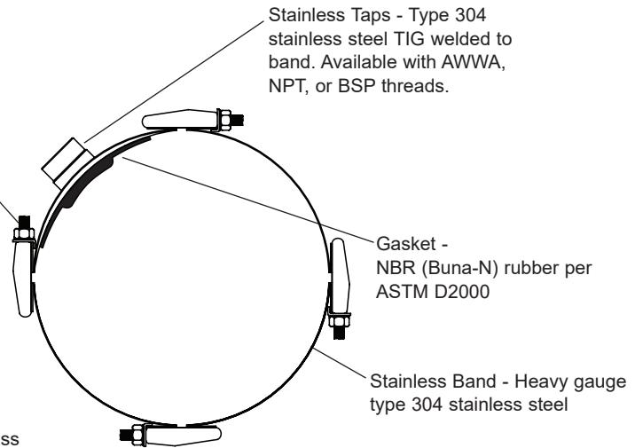
Stainless Taps - Type 304 stainless steel TIG welded to band. Available with AWWA, NPT, or BSP threads.
