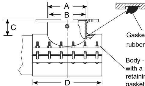
Gasket - NBR (Buna-N) rubber per ASTM D2000
