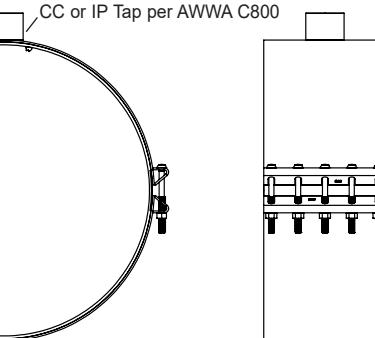
Bolts, Nuts, & Washers - Type 304 stainless steel per ASTM A193 and A194. Heavy hex nuts and washers are coated to prevent galling and maximize bolt efficiency.
