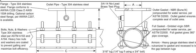
Full Gasket - Gridded virgin SBR compounded for water service, per ASTM D2000. Full gasket gives 360°
