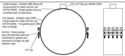
Bolts, Nuts, & Washers - Type 304 stainless steel per ASTM A193 and A194. Heavy hex nuts and washers are coated to prevent galling and maximize bolt efficiency.
