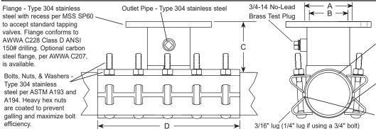
Outlet Gasket - NBR (Buna-N) compounded for water service, per ASTM D2000. Outlet gasket ensures complete seal of outlet area.
