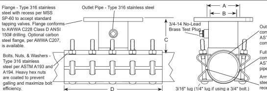
Outlet Gasket - Virgin NBR (Buna-N) compounded for water service, per ASTM D2000. Outlet gasket ensures complete seal of outlet area.
