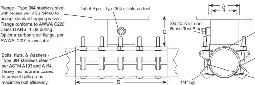
Outlet Gasket - NBR (Buna-N) compounded for water service, per ASTM D2000. Outlet gasket ensures complete seal of outlet area.
