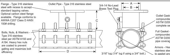
Outlet Gasket - Gridded NBR (Buna-N) compounded for water service, per ASTM D2000. Outlet gasket ensures complete seal of outlet area.
