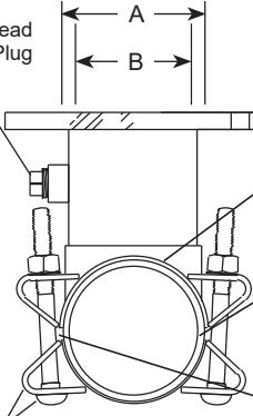
Outlet Gasket - Gridded NBR (Buna-N) compounded for water service, per ASTM D2000. Outlet gasket ensures complete seal of outlet area.
