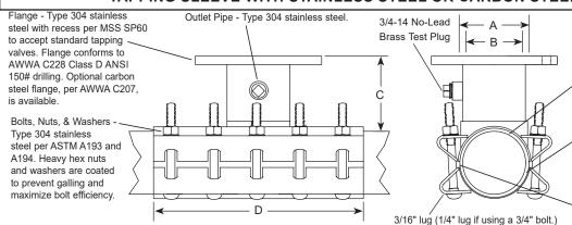
Outlet Gasket - Virgin NBR (Buna-N) compounded for water service, per ASTM D2000. Outlet gasket ensures complete seal of outlet area.
