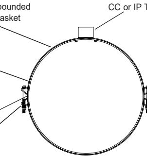
Bolts, Nuts, & Washers - Type 304 stainless steel per ASTM A193 and A194. Heavy hex nuts and washers are coated to prevent galling and maximize bolt efficiency.
