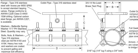
Outlet Gasket - NBR (Buna-N) compounded for water service, per ASTM D2000. Outlet gasket ensures complete seal of outlet area.
