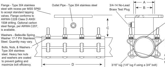
Outlet Gasket - NBR (Buna-N) compounded for water service, per ASTM D2000. Outlet gasket assures complete seal of outlet area.
