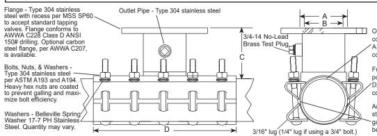
Outlet Gasket - Virgin NBR (Buna-N) compounded for water service, per ASTM D2000. Outlet gasket assures complete seal of outlet area.
