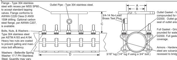
Outlet Gasket - Virgin NBR (Buna-N) compounded for water service, per ASTM D2000. Outlet gasket ensures complete seal of outlet area.
