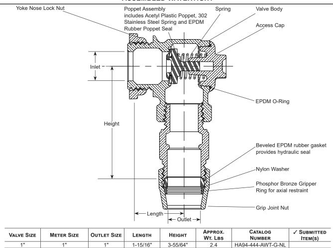
Drain/Test Valve available - add "D" to catalog number
