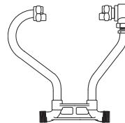
METER NUT BY ANGLE DUAL CHECK VALVE (5/8" X 3/4" METER)
