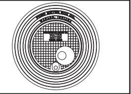
FLAT LOCKING COVER WITH PLASTIC LID WITH RECESSED HOLE FOR EMRM
