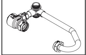
METER NUT INLET BY DUAL CHECK VALVE OUTLET (5/8" X 3/4" METER)
