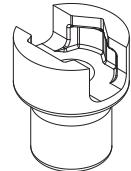
KEY SOCKET FOR STANDARD PENTAGON BOLT WITH SLOT
