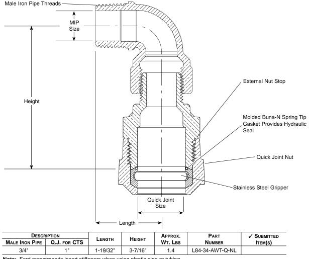
Note: Ford recommends insert stiffeners when using plastic pipe or tubing.
