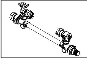
ANGLE BALL VALVE BY ANGLE DUAL CHECK VALVE WITH SADDLE NUTS
