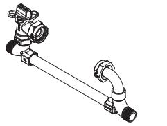
ANGLE KEY VALVE BY METER NUT (5/8" X 3/4" METER)
