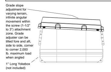
Direct loading legs for horizontal mounting rests on box top, 10,000 lb. maximum load, 1-1/2" rise
