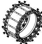
14" - 36" RESTRAINED COUPLING FOR AWWA C900, C909 OR HDPE PIPE
