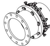
RESTRAINED ADAPTER FOR CONVERTING PLAIN END PIPE TO A FLANGE CONNECTION FOR DUCTILE IRON PIPE
