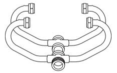
TYPE B - PLACES 3/4" METER(S) OR SECOND DEVICE IN PARALLEL POSITION
